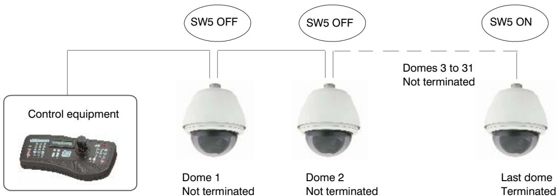
Figure 1-3 RS485 Daisy-Chain Wiring (up to 32 domes): Control in the Middle
